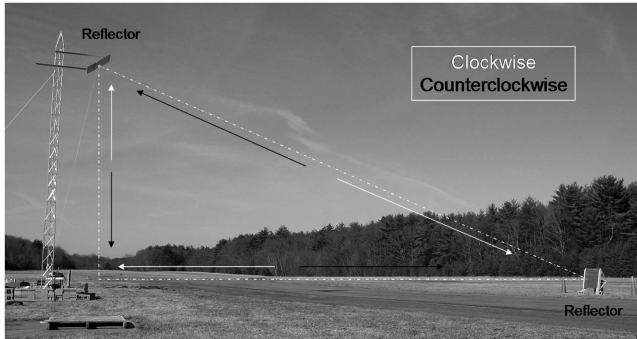
Fig. 3 Test equipment setup showing directions of signal transmission.
